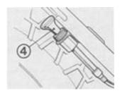
After adjusting preload air pressure, set the front and rear rebound damping adjusters (reference: (3) front; (4) rear) to one of three positions for the front and three positions for the rear. Adjust damping to provide the desired ride according to the chart below.
