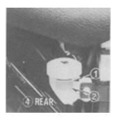
The brake fluid level in the reservoir must be maintained between the upper (1) and lower (2) level marks. Whenever the level falls near the lower level mark (2), check the brake pads for wear (see Brake Pads below). If the brake pad wear does not exceed the limits, this will usually indicate a fluid leak. Consult your nearest Honda dealer.
